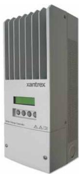
The XW-MPPT60-150 can be used with PV arrays with voltages ranging from battery voltage to 150 VDC and can support an output of up to 60 amps into the battery for battery voltages of 12 to 60 VDC. The PV open circuit voltage must not exceed 150 VDC.
