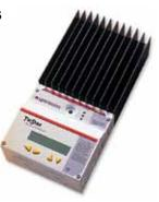
Two models are available with UL current ratings of 45 and 60 amps. A choice of 7 different set points are easily selectable with DIP switches. An RS-232 communications enables PC connection to adjust control set points and data logging. An optional digital display may be mounted on the front of the controller or up to 100 feet away using 4-conductor phone cable with RJ11 jacks.
