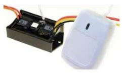
15-amp and 40-amp versions are available. Controllers have a motion sensor to activate the light or load when motion is sensed. They have temperature compensation and can be used with sealed or flooded batteries. Pulse action reduces sulfation.
