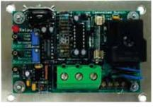
rises to the high set point. The relay in the "Active-Low" is powered when voltage drops to the low set point. The SPDT relay allows the voltage controlled switch to either connect or disconnect a circuit when it operates or to turn one thing on while turning another thing off.
