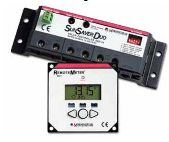
The SunSaver Duo 2-battery controller for RVs, caravans, boats and cottages is rated for 25 amps at 12 volts DC. This product will charge two separate and isolated batteries at the same time, such as a house and an engine battery, based on user selectable priorities. The SunSaver Duo employs Morningstar's SunSaver controller technology, whose long-term track record for high reliability and improved battery charging is well-recognized in the solar industry.
