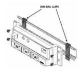
SunSaver controllers and to either snap on to the middle of the rail or to slide on from the end of the rail. The DIN rail clips are compatible with the SunSaver, SunLight, SunSaver Duo, and SunSaver MPPT.
