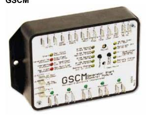
The GSCM (generator start controller module) is a microprocessor-based generator-starting controller that receives start commands from the 12-volt output from an OutBack FX inverter auxiliary relay, a user-supplied switch, an auxiliary relay in an inverter, a voltage controlled relay, a timer or any user-supplied contact closure. It automatically controls a gas/propane or diesel powered generator or pump, and is totally sealed for harsh environment operation.
