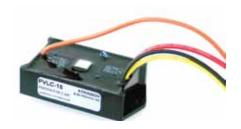
Available in 15-amp and 40-amp versions, controllers have low-voltage load disconnect and temperature compensation and can be used with sealed or flooded batteries. Pulse action reduces sulfation.
