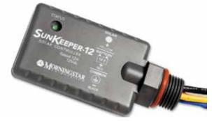
The SunKeeper is available in 6-amp or 12-amp versions at 12 volts DC. To withstand the high temperatures at the solar module, the controller has been designed using extremely efficient power electronics and is rated to 70C. The SunKeeper is also certified for use in Class 1, Division 2 hazardous locations, making it an ideal controller for solar powered oil/gas applications. Mounts in 1/2" knockout.
