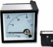
These high quality amp meters mount in a 72mm square hole. The meter movement is very smooth and accurate. The shunt is built into the 30-amp meter so it can be in series with the load to be measured on the negative or positive wire. The 60-amp meter comes with a separate shunt. The mounting plate in the table below holds 1 meter and mounts in a 2-gang wiremold deep switch box.
