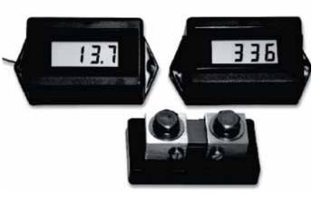
Measure amps and volts in 12-, 24- or 48-volt systems with these high-quality, low-cost LCD digital meters. The surface mount, 3" x 2" x 1" plastic enclosure can be attached to wood or metal surfaces with two screws. Terminal strip on the back of the meter accepts 14 to 22 AWG wire.
