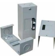
The Big Baby overcomes the Baby Box smallness. This box is at least one inch larger in all dimensions. It also includes a ground box lug and mounting provisions for our short insulated busbar. It holds up to 4 of the 13mm wide DINrail breakers from 1-63 amps. Box Size is 9" x 5" x 4" and weighs 3 pounds.
